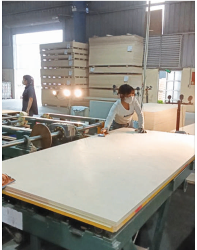
Minor patching after sanding.
