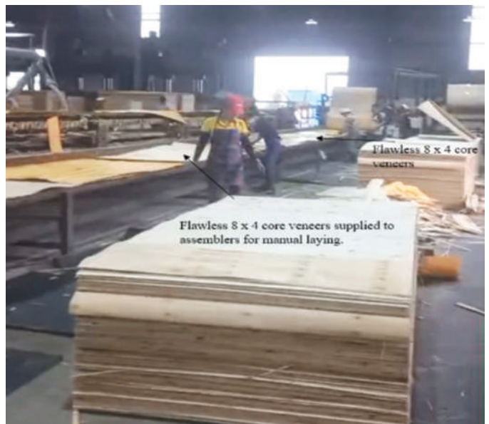
8 x 4 core veneers for manual laying on the base veneer.
