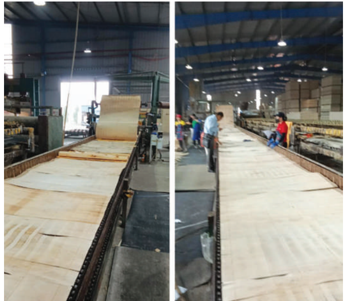
Assembling lines with veneer rolls (for top and bottom layer).
