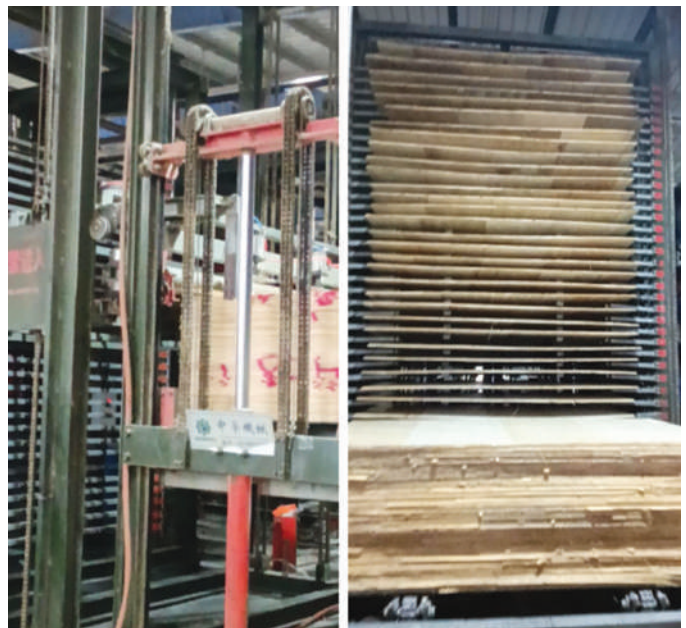
Hot press with automatic loader and unloader.
