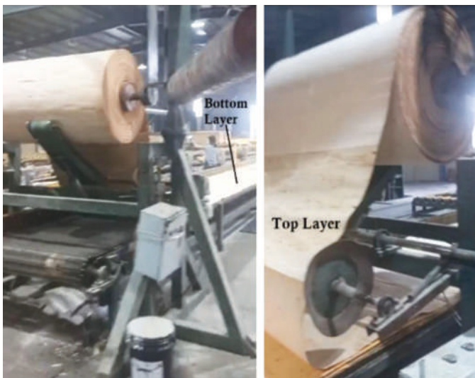
Rolls supplying bottom and top layer of the mat.
