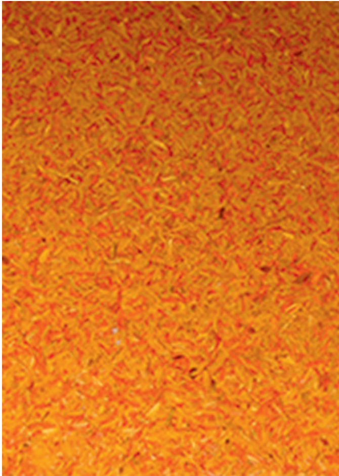
Figure 2: Rice husk Particle Board.
