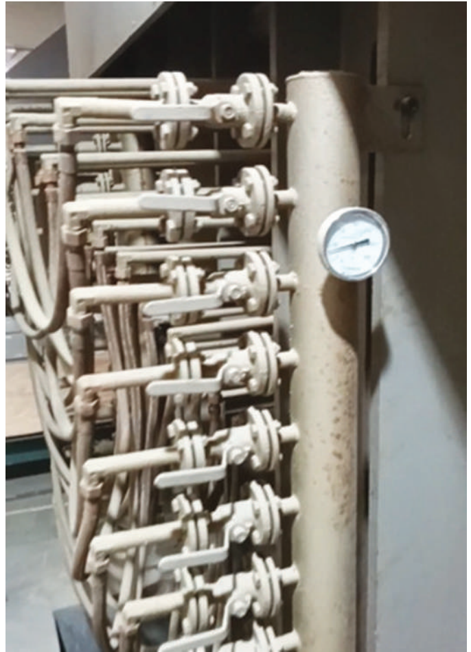
Hot press equipped with individual inlet and outlet valves.
