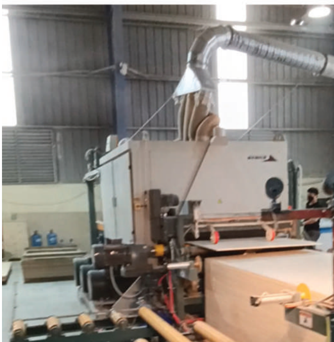
Trimming and Sanding
