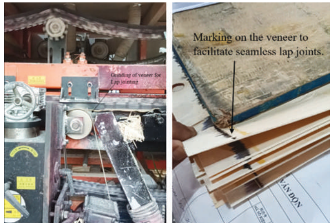
Grinding of veneer edge for lap jointing and marking for seamless joint.
