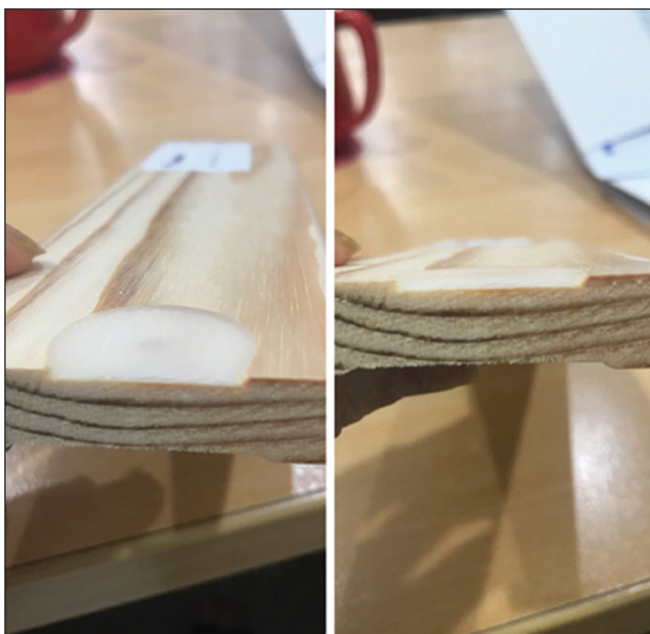
Repaired with colourless Teknos Uvilux Putty 1465-00
