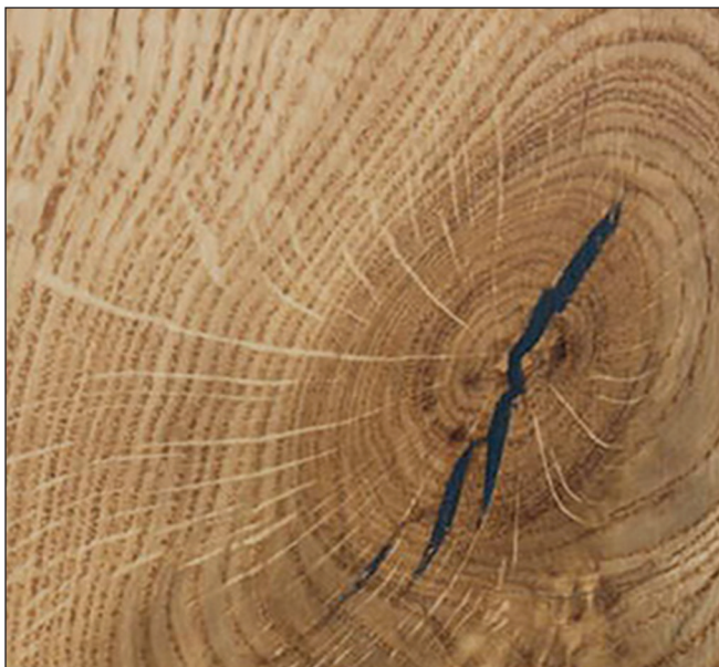
Repaired with pigmented Teknos Uvilux Putty 1465-20
