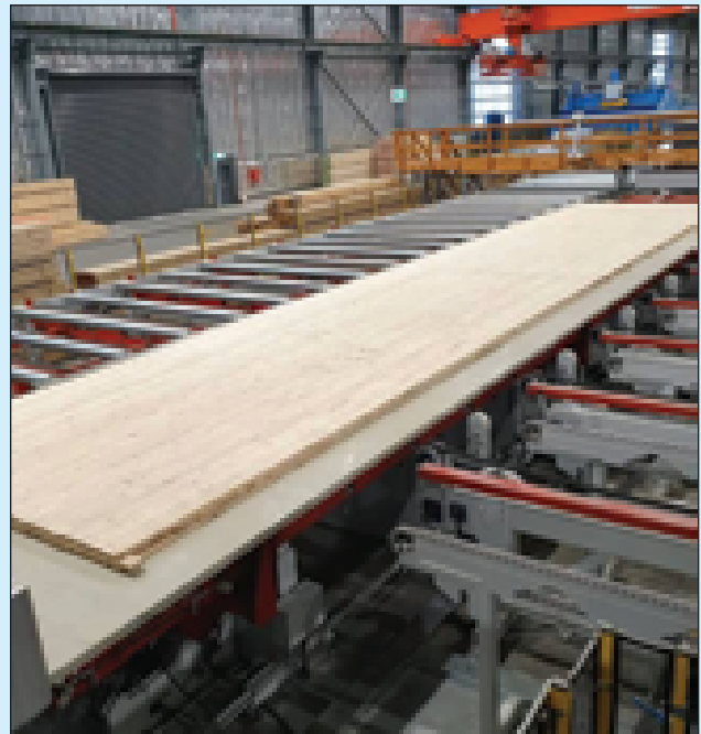
The first CLT panel pressed at the NeXTimber facility.
