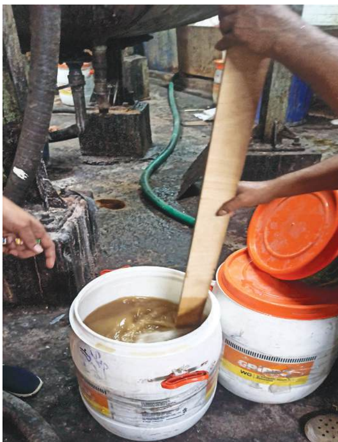
Soya urea melamine formaldehyde resin on 2nd day of cooking and its flow property in B4 cup.
